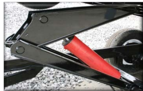
HT-514 scissor hoist (5" bore x 20" stroke)
