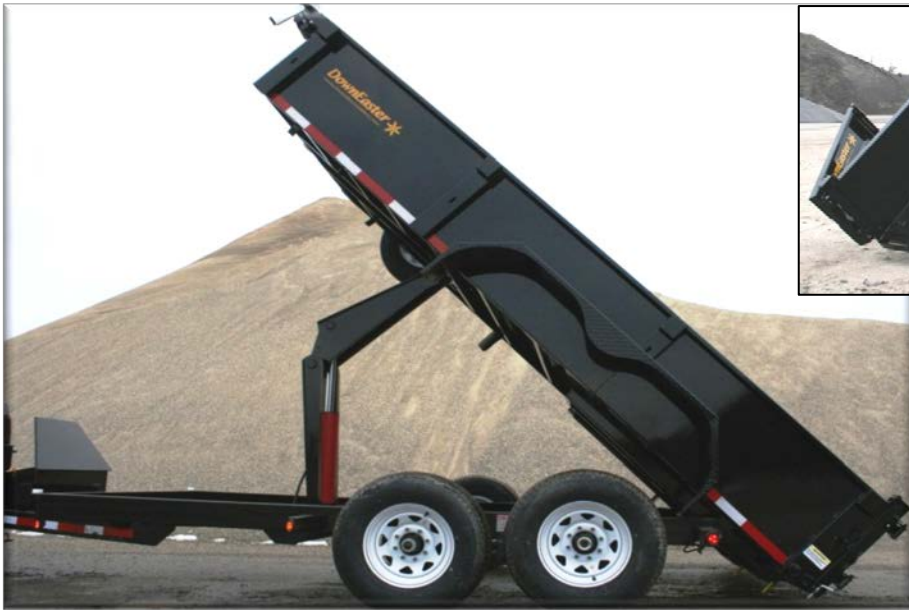
HT-514 Scissor hoist with 5" x 20" cylinder, provides a more stable center load lift and less body twist, than dual cylinders.
