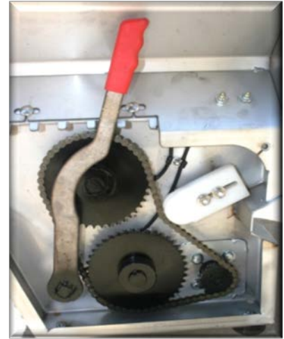
Enclosed, chain drive gear case
