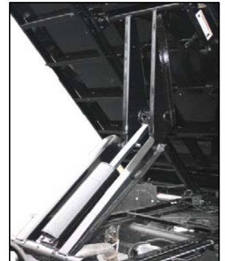
HD-512 scissor hoist, 5" bore x 16" stroke
