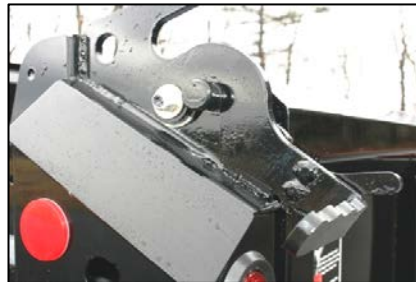
One handed, self aligning, locking latch w/ integrated spring retention
