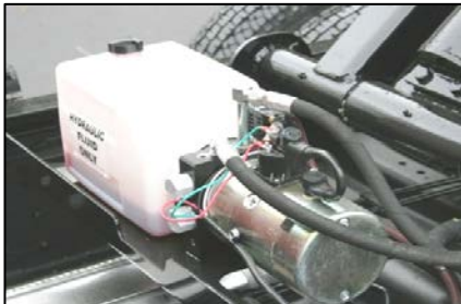
Dual action pump, shipped installed
