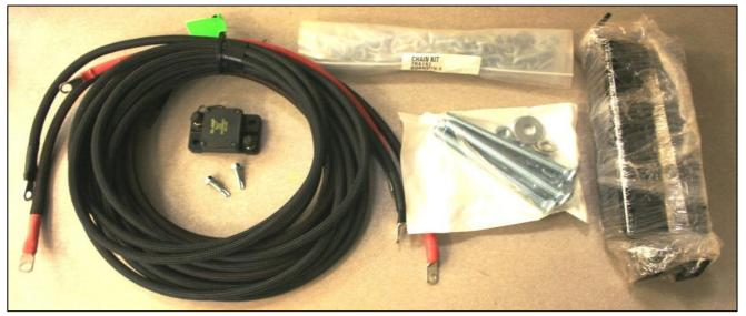
NOTE: some short bed Dodge ram trucks from 2003 to 2009, may require an extension kit, due to the bed length of 6'-4", being 2" short of nominal length for proper clearance.
