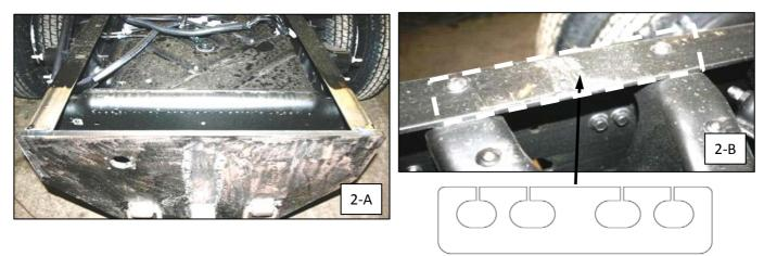
On certain brands of trucks, some electronic modules, located on cross members, may need to be relocated, as to not interfere with the scissor hoist mounting location. (example: GM modules shown
