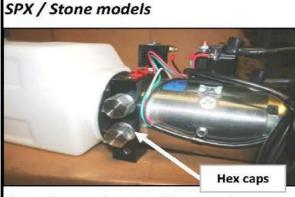
The two hexagonal caps <u>must be removed</u> to access pressure screw.
