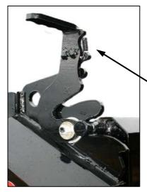
Move latch handle up and lock latch into stored vertical position. DO NOT STAND DIRECTLY BEHIND GATE WHEN LOADED.
