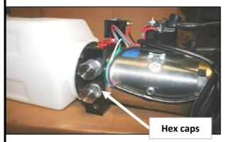
The two hexagonal caps <u>must be removed</u> to access pressure screw.
