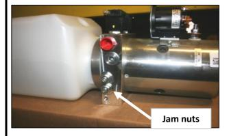
The two 9/16" wrench size jam nuts, <u>must be loosened</u> to access the 3/16" Allen head pressure screw.
