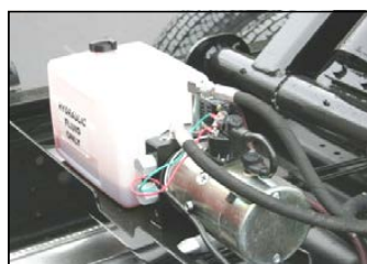
Dual-action Pump, Installed
