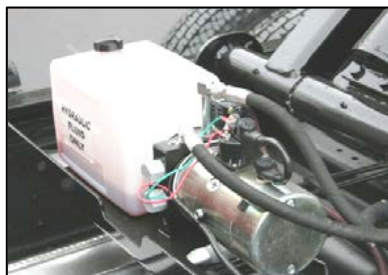
Dual-action Pump, Installed
