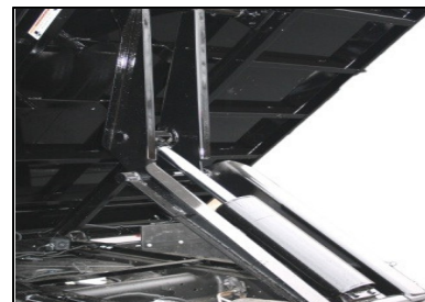
Champion Hoist, Installed
