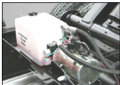
Dual-action Pump, Installed
