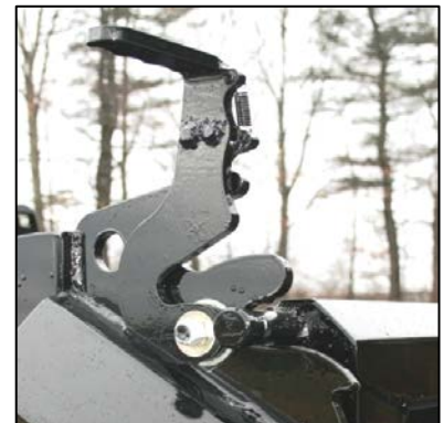
One handed, self aligning, locking latch w/ integrated spring retention
