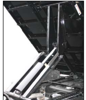
HD-512 scissor hoist, 5" bore x 16" stroke
