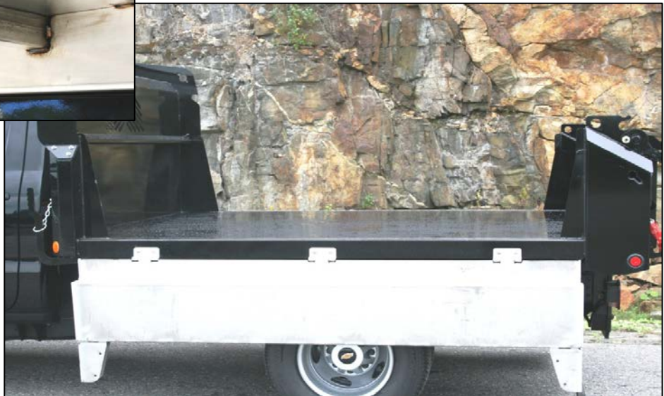
HD-512 scissor hoist, 5" bore x 16" stroke
